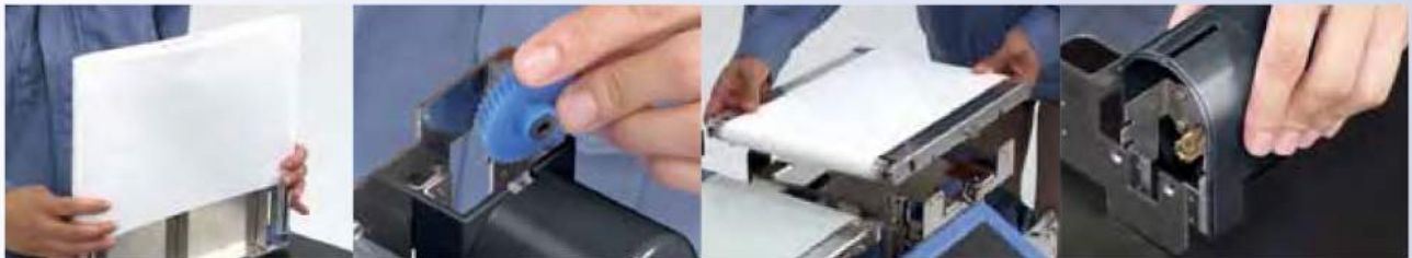
Replacing a belt
